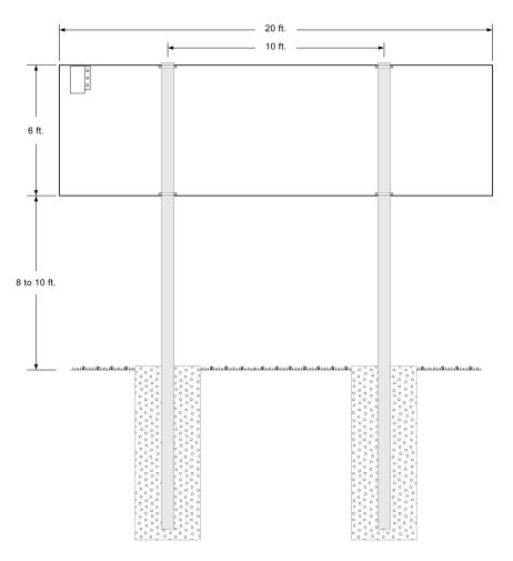
Once you have verified the positions of the posts and the size of the footings, you are ready to dig your holes, pour your concrete, and set your posts. There are several techniques for ensuring proper alignment of the posts. Typically installers will construct a temporary wooden support frame to hold each post in place while the concrete sets. Having plumb posts in the proper position is the key to a smooth mechanical installation.
